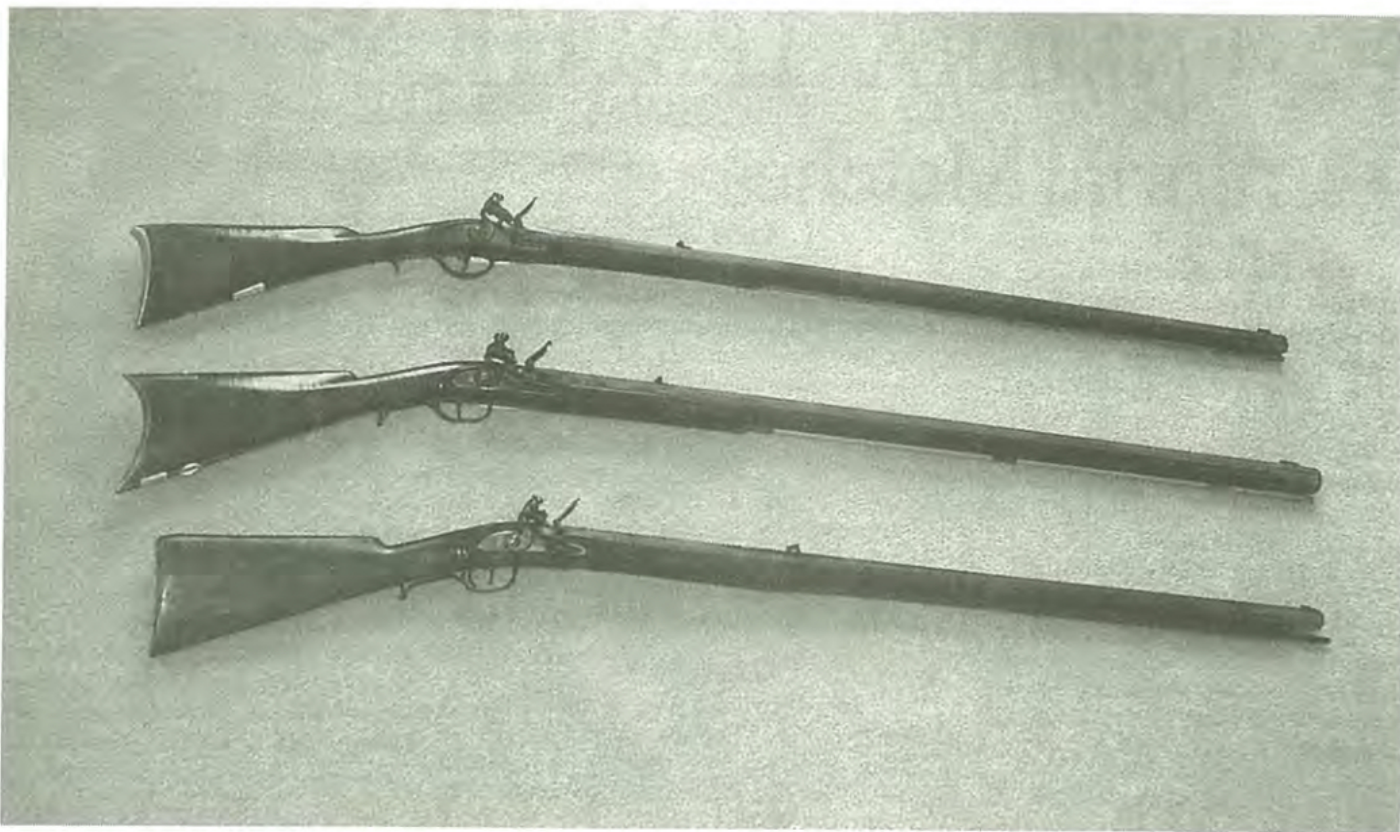
Three traditional styled fullstock chunk guns. Top: brass mounted Lancaster 1" x 48" .45 caliber; middle: iron mounted Tennessee 1 3/16" x 48" .50 caliber; bottom: iron mounted 1 1/8" x 46" .45 caliber. This gun is ugly, but it has set several records on the chunk line at the NMLRA Nationals in Friendship, Indiana.
