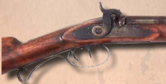
S. Hawken trigger guard and snail (Courtesy of Gordon, 2007)
