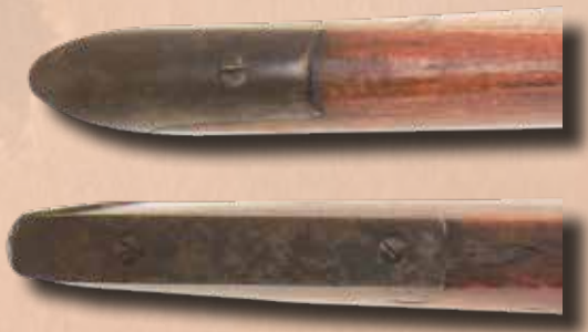
Toeplate and buttplate extension on original rifle (Courtesy of Gordon, 2007)
