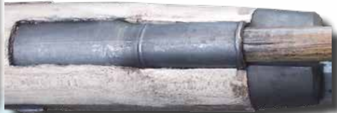
Rear thimble and nose cap installed.
