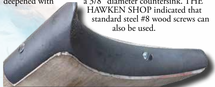
Butt plate installed.
