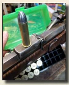
Casting 30-1 lead/ tin, my bullets were weighing in at 520 grains at an 825 degree pour.
