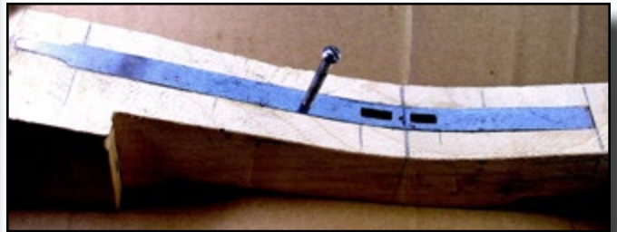
Fig. 4. A tightly fitting mortise can make you a victim of your own success. Luckily you can back out the plate by turning a #10-32 screw down through the mainspring screw hole against the bottom of the mortise. Trying to pry out a long inlay like this can wedge it deeper into the mortise if what you do straightens the inlay. Note that the plate swells a bit forward of the trigger slots. That can be removed by filing down to wood level to match the smooth curvature of the wrist.
