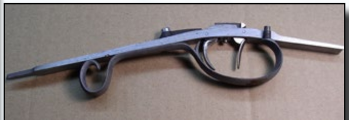
Fig. 5. Leaving a 1/8" of free play behind the rear trigger gives plenty of room up front for a gloved finger. I love that straight, early style grip rail that hugs the plate to give plenty of solid gripping area. It appeared frequently on both fullstocks and halfstocks during the J&S period. (Baird 2)
