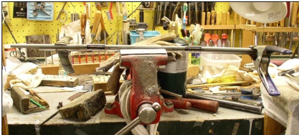
Fig. 21. The rib is held in the vise between padded inserts. The ends of the all-thread rod are clamped down into the rib's ramrod groove to center the thimbles on the rib flats. Now to clean up my workbench...
