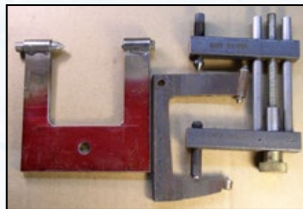
Fig. 10. Two versions of my drill guide, consisting of a pilot concentric with a point, are shown on the left. Scott Coy's improved guide is on the right. All are adjustable, but the one in the middle is most suitable for drilling holes for patchbox latch pushrods.
