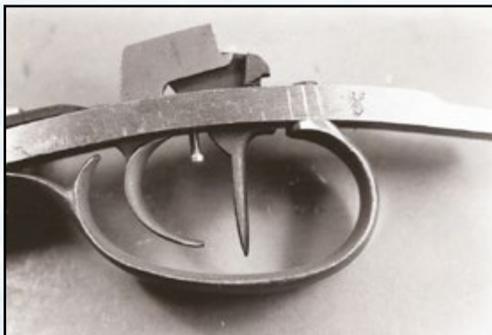
Fig. 8. There! That's a nice tight fit flush against the plate with no free play.
