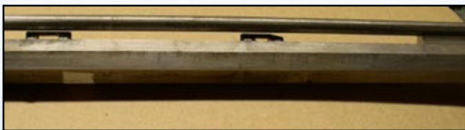
Fig. 12. By clamping a straight 3/8" diameter rod in the rib groove, you can tell how much ramrod clearance you will have over the lugs. Note that I filed off a corner of the forward lug to clear the full cast return thimble (described in Fig. 18).
