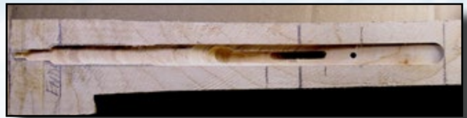
Fig. 3. The milled trigger plate mortise still needs a bit of handwork, but at least 95% of the wood has been removed. During removal of the remaining wood, that gives it some place to go... a big factor when cutting a deep, long mortise.
