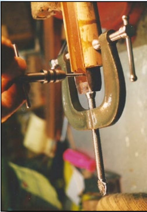
Fig. 15. The only effective way to press a cap to full, sustained contact against the forestock shoulder is to apply a three-pad edging clamp. If AcraGlas or other epoxy bedding agent is not used to secure the cap, thread in a flat head #2-56 machine screw.
