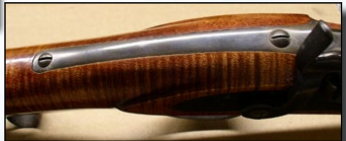
Fig. 9. For best appearance, these screws must be aligned properly through the long Hawken tang.
