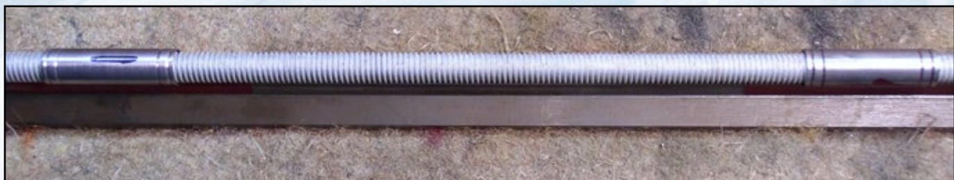
Fig. 20. All-thread rod serves a dual purpose of alignment and clamping pressure without drawing away a lot of heat during soldering.
