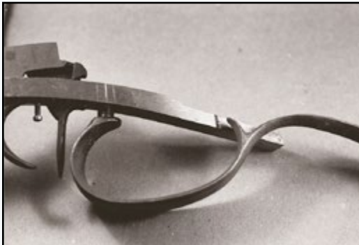
Fig. 7. Nope, it isn't going to turn in tight unless you solve the interference from the front end of the plate.
