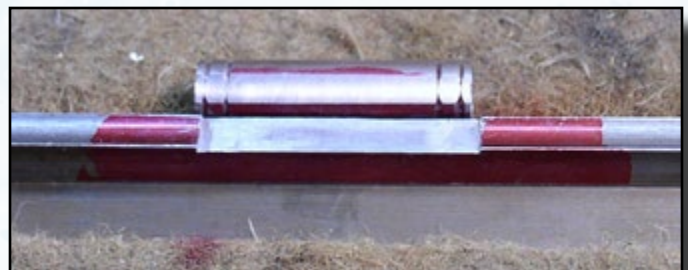
Fig. 19. The final stage of rib installation is thimble attachment. Note that the thimbles have been turned to match the cast entry thimble and milled to match the flats on the rib. The red lay-out dye provides a contrast to keep old eyes from making mistakes.
