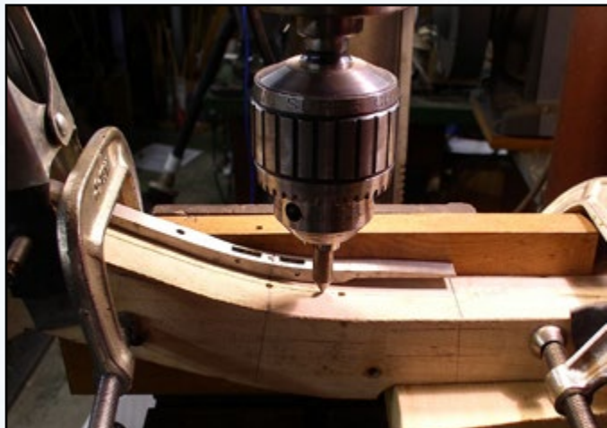
Fig. 2. The massive angle plate has been faced with a board to prevent stock contact with its much-abused surface. A centerpoint mounted in the drill chuck is the only reliable way to index on the centerline of the stock. I do a dry run along the whole length of the line to make sure the milling table travel is indexed to it.
