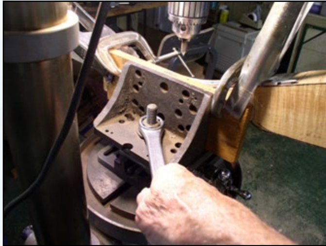
Fig. 1. The position of the plate can be adjusted by loosening the T-bolt lockdown so that the milling table travel follows the stock centerline precisely over the whole length of the trigger mortise.
