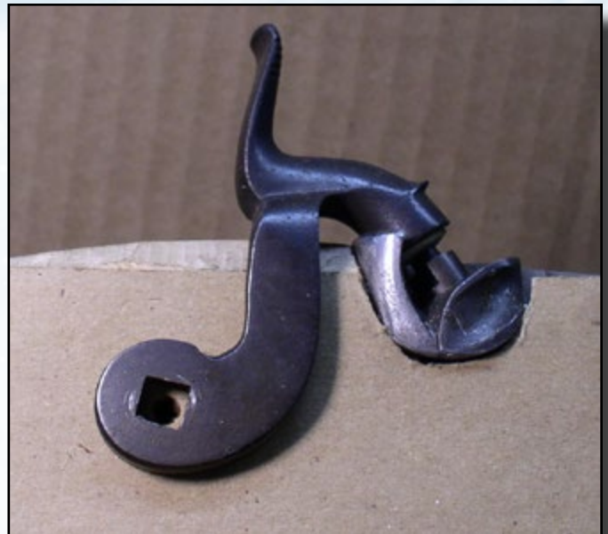
Fig. 11. Here is a mock-up of the positioning of the hammer on the panel while its nose is centered on the nipple. I got so carried away with inletting the lock plate that I forgot to take this picture in a timely fashion, but Keith Lisle reminded me. It is good to have an editor who knows more than the author...
