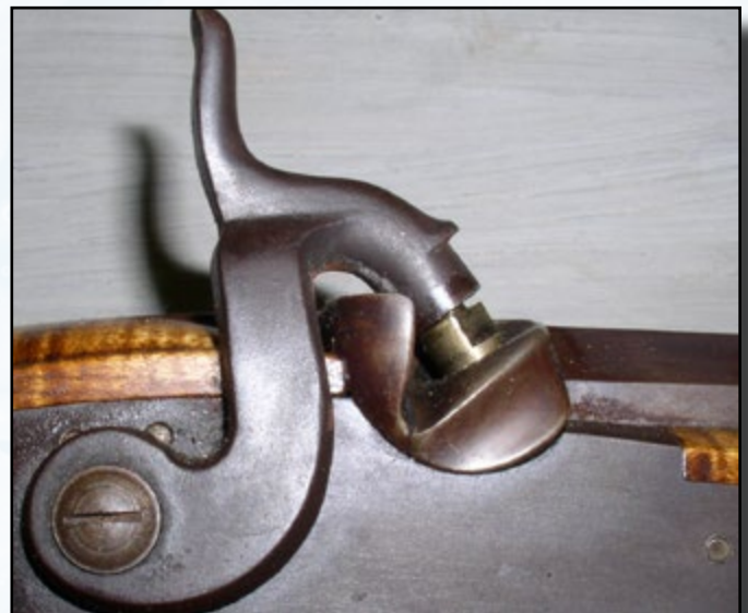
Fig. 8. Good metal-to-metal fit is not only aesthetically pleasing, it is necessary to keep percussion cap flash from depositing corrosive chemicals in the lock mortise. Note the rust piling up on the side of the barrel just forward of the breech. As an after-thought, increasing the depth of the hammer cup reduced the blow-by and allowed the hammer to square with the nipple.
