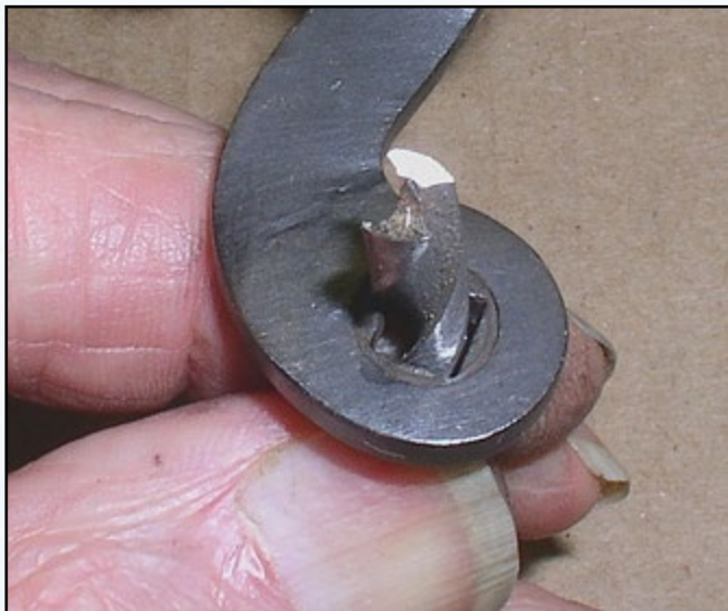
Fig. 10. This 15/64" brad-pointed wood bit is just right to center-mark through the tumbler hole in the hammer. Just make sure that the hammer nose stays securely centered on the nipple.
