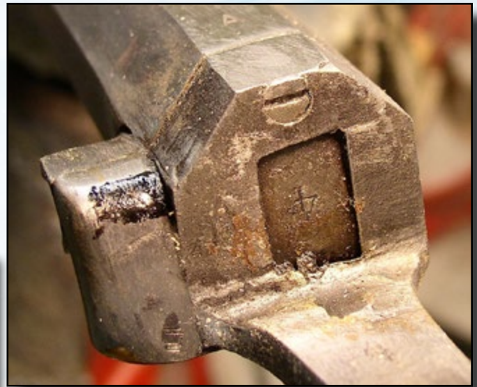
Fig. 7. Seldom does the cast breech plug fit the scallop of the lock plate, so now it is file-and-fit time using inletting black. Note the #3-48 screw holding the parts tightly together.
