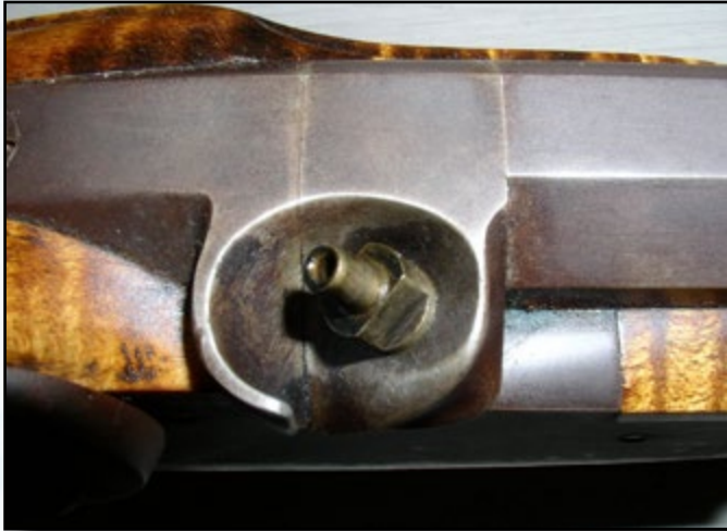
Fig. 6. A well fitted breech mates tightly in every dimension including the circumference of the nipple recess. The browning along the mating surfaces did not take well because of grease leaching from between the parts. Better degreasing before browning would have prevented this problem.
