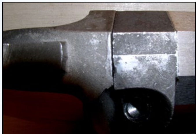
Fig. 2. Badly cast parts and mismatched plug/standing breech assembly are impossible for the first time builder to rectify.
