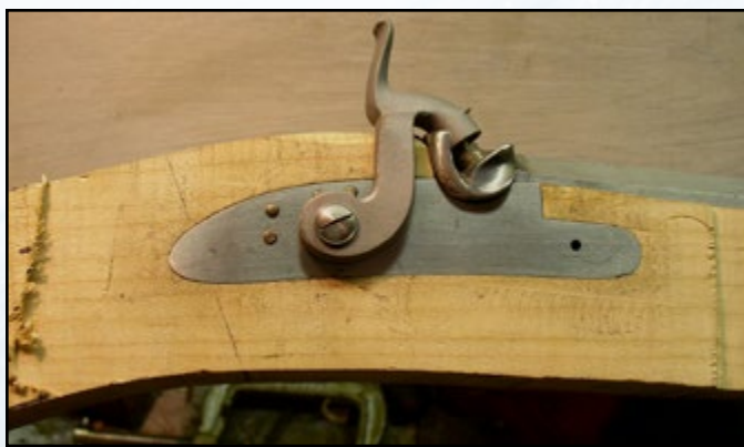
Fig. 13. This line indicates the approximate angle of sear arm travel. A lot of wood still needs to be removed from the belly/wrist area before inletting the trigger plate.
