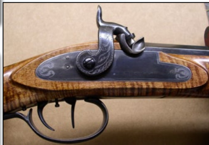
Fig. 4. As in every muzzleloading rifle, the wood-to-metal and metal-to metal fit proclaims the competence of the builder. Note the faucet washer to protect the nipple during dry-firing the rifle.
