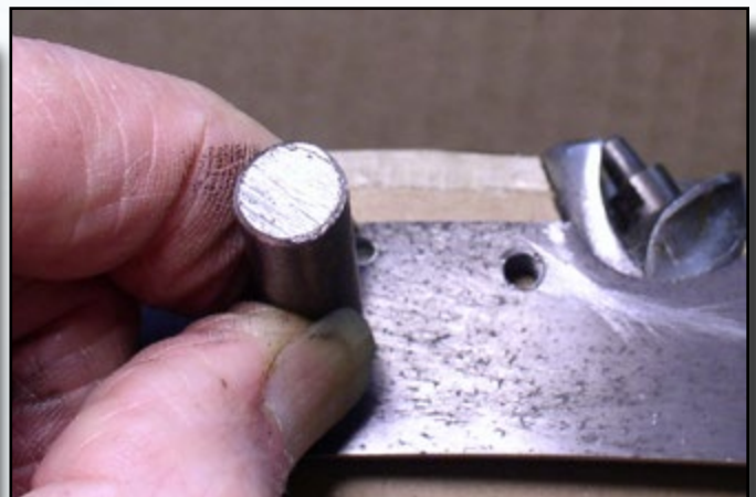
Fig. 12. Here I am inserting the locator tool (shown in Fig. 9) through the lock plate's tumbler hole into the hole in the panel.
