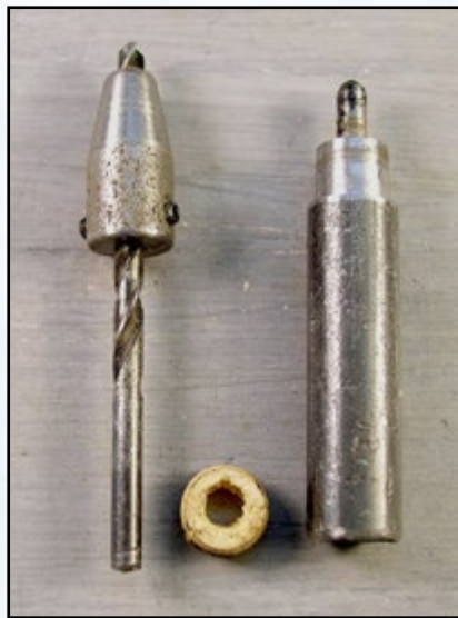
Fig. 9. Hawken-specific tools left to right: a drill stop to prevent drilling into the bore when installing the underrib, a hammer cup insert (no, it's not a Cheerio!) to ensure accurate alignment between hammer and nipple and a lock-positioning pin to be inserted through the tumbler hole in the plate. The drill stop on the left will be absolutely essential for the under-rib installation in Part II.
